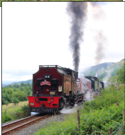
Two Garrett's re-starting a 20 car 300ton train on 1:40 with Columbian smoky coal and our own John Shawe at the controls of the 2nd engine.
